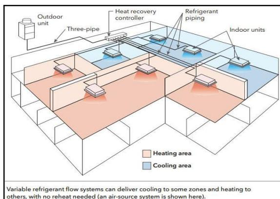
Figure 8 – Typical VRF Schematic Diagram
